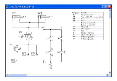
The parts list component analyzes all components of the diagram and generates table with columns for the component identifications and the component designations. In this connection, FluidSIM uses existing labels and texts as component identifications.
