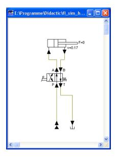
After the cylinder has been extended, the pressure in the cylinder supply line must inevitably increase. This situation is recognized by FluidSIM and the parameters are recalculated; the pressure downstream of the pump unit increases to the value, as defined by the pump unit safety guard.
