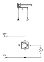
At the output the displacement encoder system provides a voltage proportional to the piston position of the interconnected cylinder. This voltage will be at its defined minimum when the cylinder is retracted completely; the voltage will be at its defined maximum when the cylinder is advanced completely.
