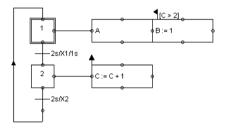
Each time step "2" is activated, "C" is raised by one. As soon as "C" has the value "3" and step "1" is activated, "B" receives value "1".
