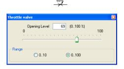
To help with precision adjustment some controllers provide an optional control range. You may alternatively enter the numeric value using the input field.
