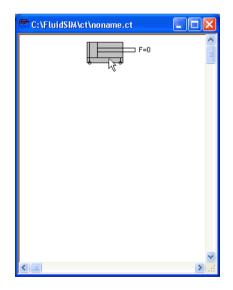
In this way it is possible to "drag" each component from the component library and place it in the desired position in the drawing area. In the same way it is possible to rearrange components already in the drawing area.
