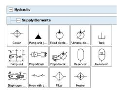
FluidSIM adds the symbol to the applicable position. The order of the other symbols will be maintained. FluidSIM keeps the symbols from being on top of each other or from creating "gaps".
