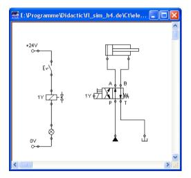
So that the valve can be controlled by the solenoid, you have to link the components with a label.
