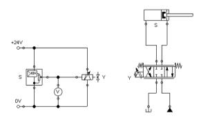
$\rightarrow$  Please launch the simulation and observe how the cylinder retracts and how the valve moves further in the closed position.
