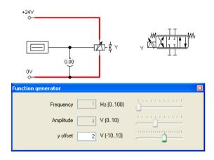
→ Gradually change the y-offset and observe how the valve moves subject to the controller setting.
