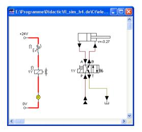
Aside from a manual or electrical operation, valves can be controlled *mechanically*, either through a cylinder piston or a magnet mounted at the piston. Such a coupling is realized in the same way an electrical coupling is established: By means of labels, which are assigned to the cylinder's distance rule and the mechanical valve connection.
