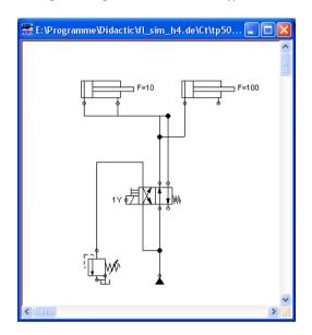
The following circuit diagram contains mistakes of type 2, 3, 4, and 6:
