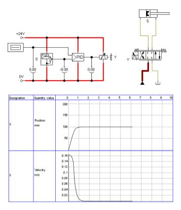
It often may be desirably to make a cylinder travel by maximum speed until it reaches its desired position, and to make it stop most spontaneously. To achieve this we can amplify the position signal of the displacement encoder and therefore accelerate the reversing of the control valve. In doing so we make use of the fact that the PID-controller limits the output voltage of the proportional valve magnet to 10 volts.
