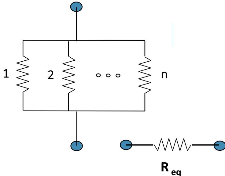
$$\frac{1}{R_{eq}} = \frac{1}{R_1} + \frac{1}{R_2} + \dots + \frac{1}{R_n}$$
