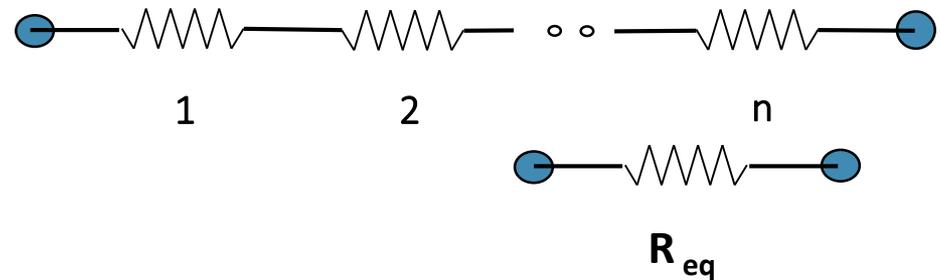
$$R_{eq} = R_1 + R_2 + \dots + R_n$$
