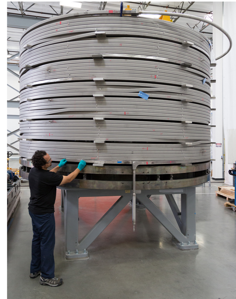
A module of the ITER CS being manufactured at General Atomics, USA
