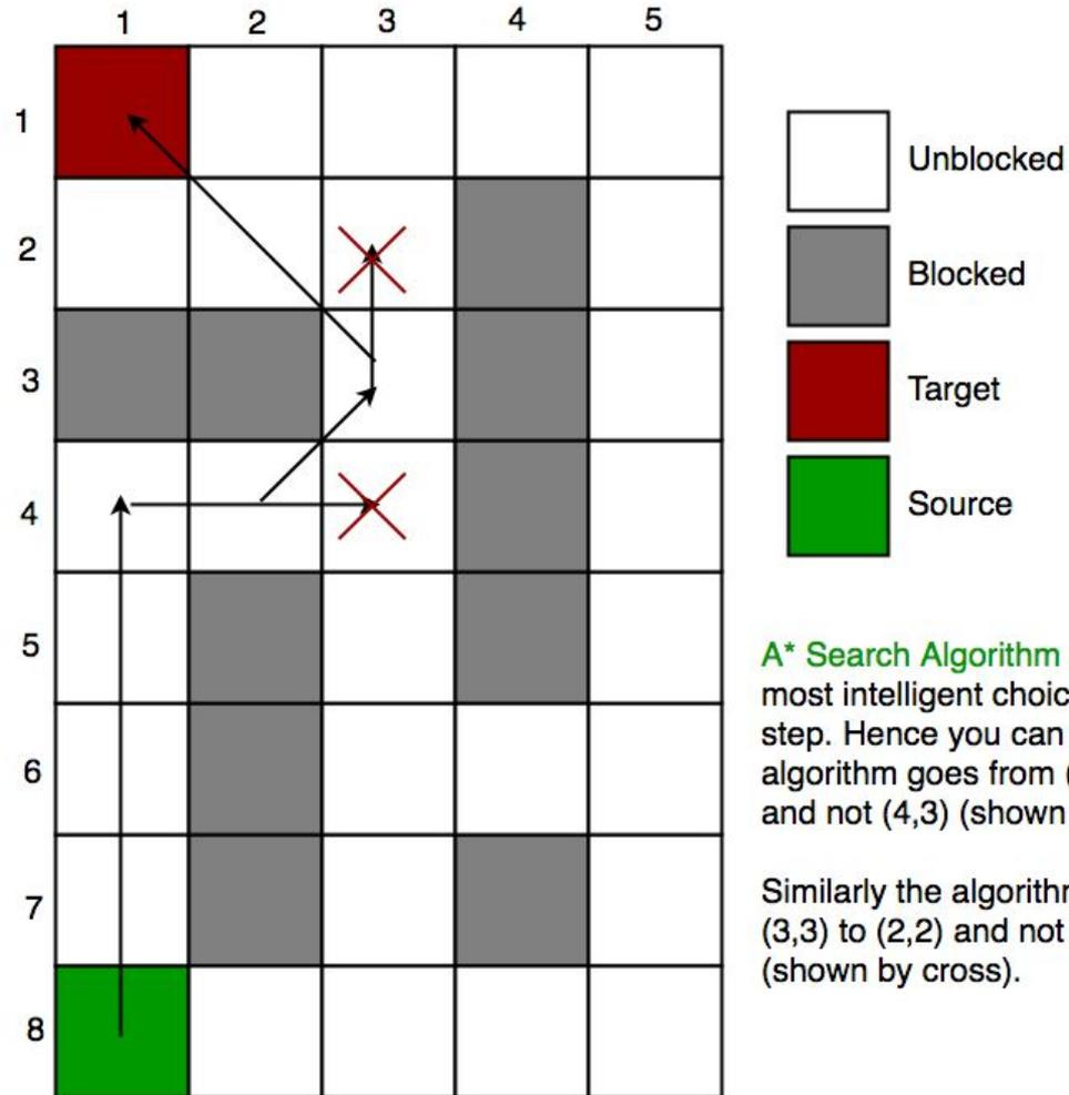
**A\* Search Algorithm** makes the most intelligent choice at each step. Hence you can see that algorithm goes from (4,2) to (3,3) and not (4,3) (shown by cross).
