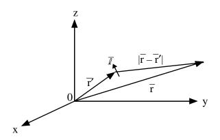
By linear superposition, the vector potential due to an arbitrary source  ${f J}$  is
