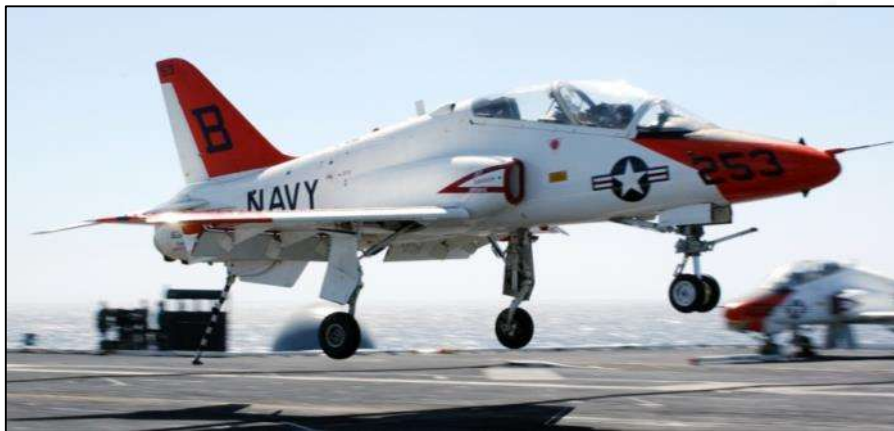
T-45 Goshawk Basic Jet Trainer – first 10 aircraft carrier landings before F/A-18 flights
