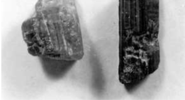
Figure 8.16 A dichroic crystal. The E -field parallel to the optic axis is transmitted without any diminution. The naturally occurring ridges evident in the photograph of the tourmaline crystals correspond to the optic axis. (E.H.)
