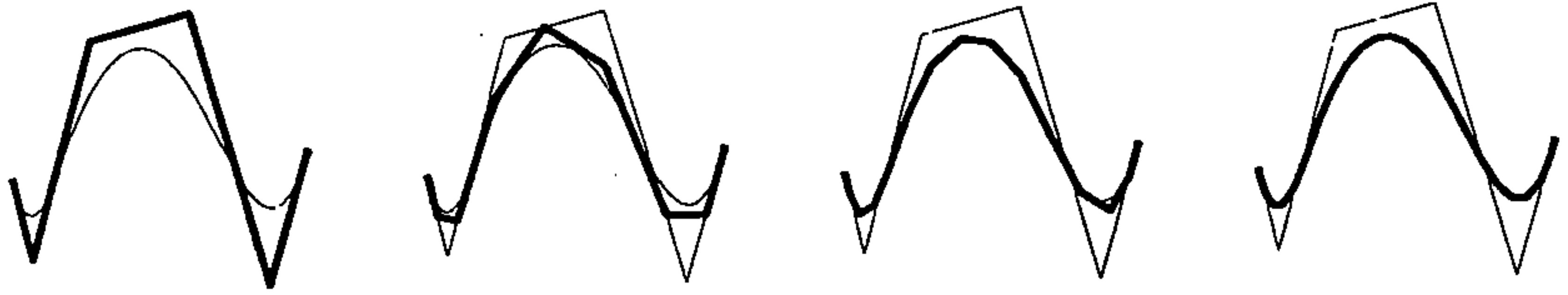
(17) FIGURE. After three midpoint refinements, the control polygon of this spline is graphically indistinguishable from the spline.
