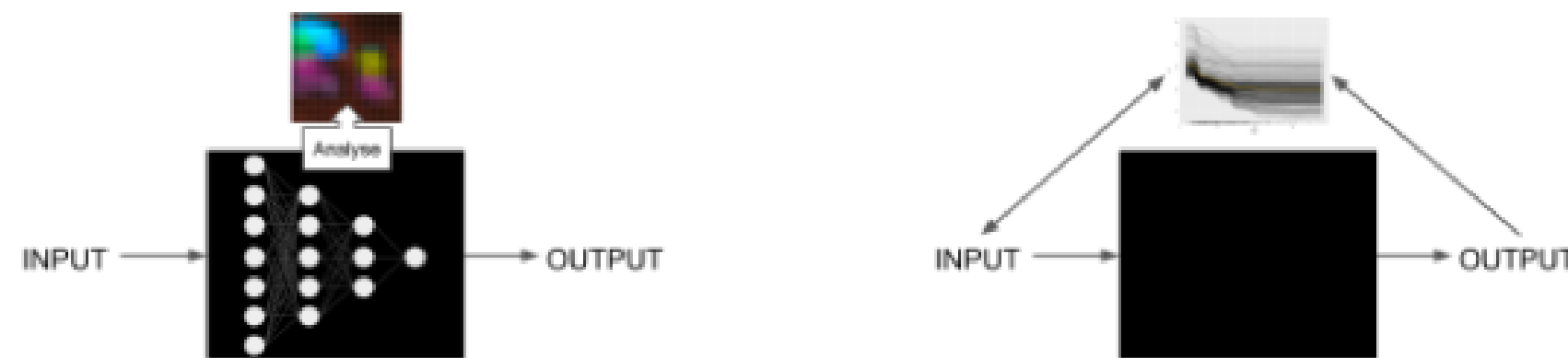
Fig. 2. Some IML approaches work by assigning meaning to individual model components (left), some by analyzing the model predictions for perturbations of the data (right). The surrogate approach, a mixture of the two other approaches, approximates the ML model using (perturbed) data and then analyzes the components of the interpretable surrogate model.
