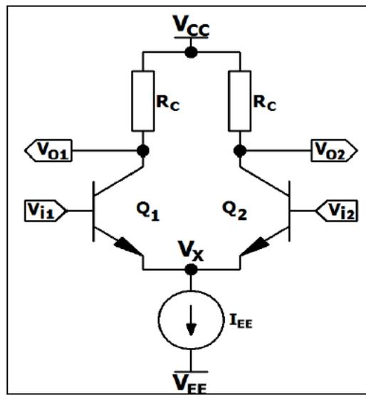
$$V_{id} = V_{i1} - V_{i2}$$
