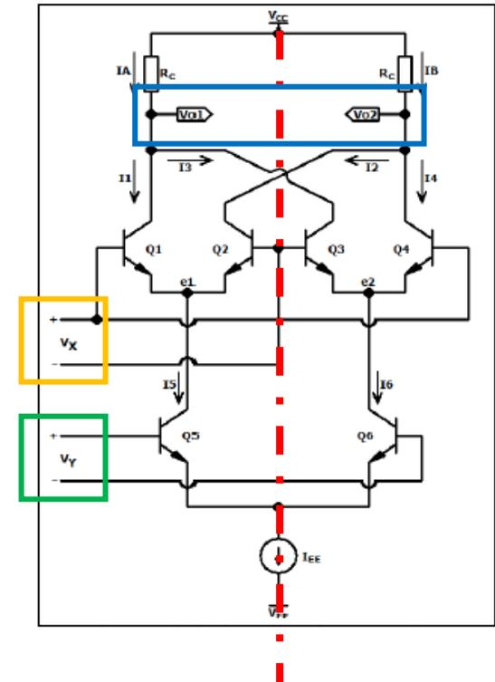
$$V_{out} = V_{O2} - V_{O1} = K V_x V_y$$
