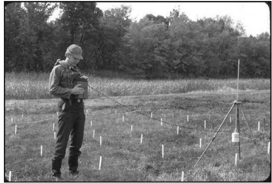
FIGURE 11.5 The layout of ground surveys involves making appropriate choices of the magnetometer, survey altitude, and grid spacing, as in this example from an archaeomagnetic survey that uses a proton-precession magnetometer at 0.5 m above the ground surface at a station grid interval of 1.5 m.
