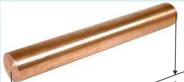
$$\frac{\partial}{\partial x} \left( k \frac{\partial T}{\partial x} \right) + \dot{q}_g = \rho c_p \frac{\partial T}{\partial t}$$
