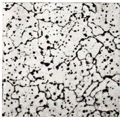
FIG. 6-5. Hypomonotectic Cu + 5% Pb alloy, as cast. Light areas are primary and monotectic Cu; dark areas are Pb which existed as L_{II} at the monotectic temperature. Magnification 100.
