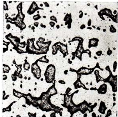
FIG. 6-4. Microstructure of cast monotectic alloy Cu + 36% Pb. Light areas are the Cu-rich matrix of the monotectic constituent; dark areas are the Pb-rich portion, which existed as L_{II} at the monotectic temperature. Magnification 100.
