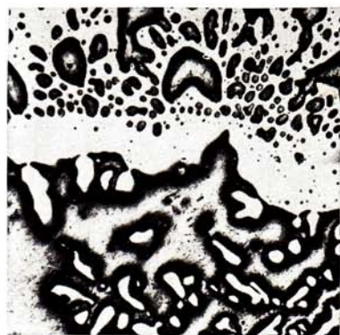
FIG. 6-6. Microstructure at the interface between the two layers in a Cu + 50% Pb hypermonotectic alloy. Upper layer is the product of the monotectic decomposition of L_I (36% Pb); lower layer contains light particles of Cu, precipitated during the cooling of L_{II} from the monotectic temperature down to that of the eutectic, embedded in the dark Pb-rich Pb-Cu eutectic constituent. Magnification 100.
