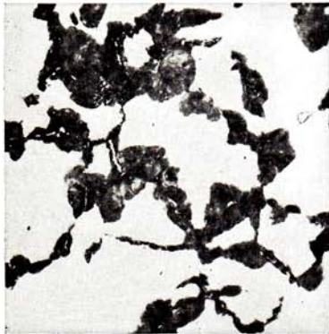
FIG. 5-12. Eutectoid steel partly transformed by cooling at an intermediate rate through the temperature range of transformation. Light areas are martensite; dark areas are partly pearlite and partly bainite. Magnification 500.
