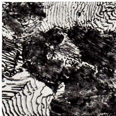
FIG. 5-11. Pearlite formed during cooling through the transformation range exhibits a wide variation in lamellar spacing. Magnification 1,500.
