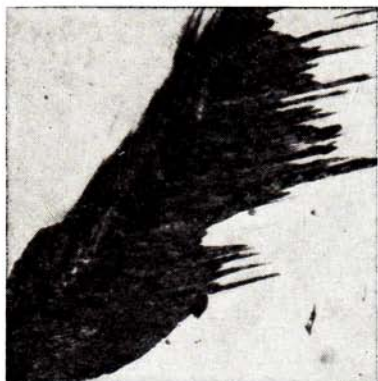
FIG. 5-7. Bainite constituent in a partially transformed carbon steel. Magnification 1,500.
