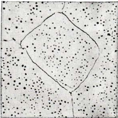
FIG. 4-17. Same as Fig. 4-13 reheated to slightly above the solidus temperature of the alloy and quickly cooled. Liquation at grain boundaries and at many isolated points within the grains has resulted in the development of a continuous film of eutectic copper solid solution at the grain boundaries and eutectic rosettes within the grains. Magnification 100.
