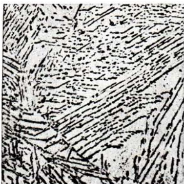
FIG. 4-14. Same as Fig. 4-13, but slowly cooled from the homogenizing temperature. Parallel platelets of copper-rich solid solution have formed upon certain crystallographic planes of the parent silver-rich solid solution, producing a Widmanstätten structure. Magnification 1,000.
