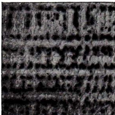
FIG. 4-12. Sterling silver (7.5% Cu) as cast. Light areas, shading from white to light gray, are cored dendrite areas, silver-rich at their centers; dark areas are divorced eutectic. Magnification 100.
