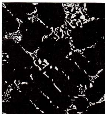
FIG. 13-9. Schematic representation of the progress of freezing of an alloy composed of 30% Pb + 5% Bi + 5% Sb, indicated by point x in Fig. 13-11. The first five pictures of the series are idealized sketches; the sixth picture is an actual photomicrograph of the alloy at room temperature. Magnification 100.
