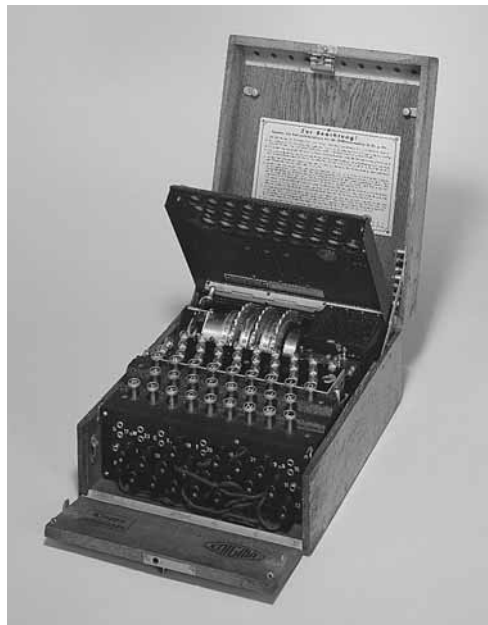
12 A three-ring Enigma cypher machine in its wooden transit case, 1930s. It was used by the Germans during WWII to encode and decode secret transmissions to U-boats.
