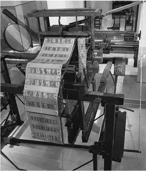
2 A Jacquard silk-weaving hand-loom, the first machine to use punched-card programming, 1810.
