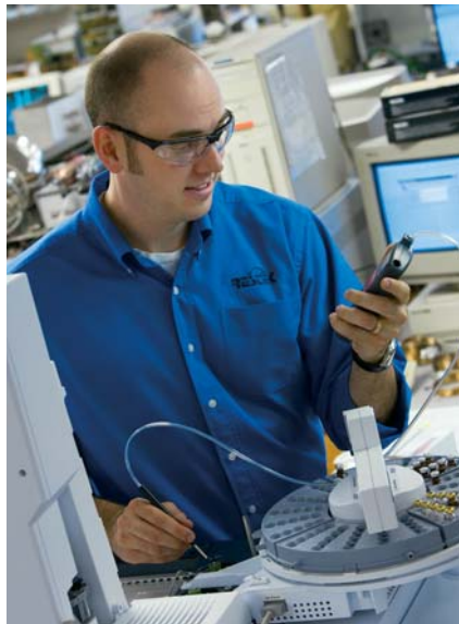
Scott Grossman, Applications Chemist Checking for leaks, using a thermal conductivity leak detector (step 13).
