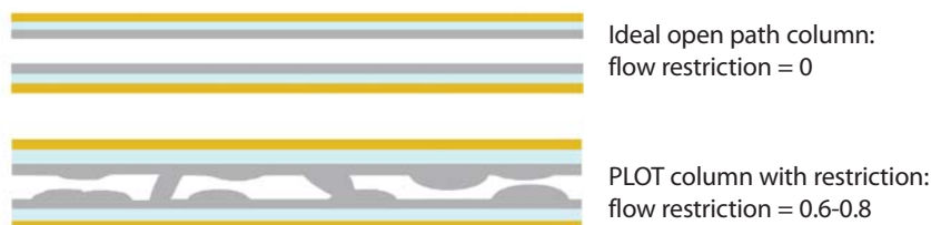
Figure 2 Inconsistent coating thicknesses result in restrictions that cause significant variation in flow.
