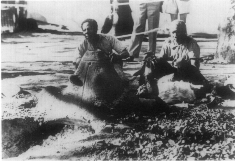
FIG. 5. A MaShona forced draft furnace built for a 1942 iron smelting demonstration in Zimbabwe.
