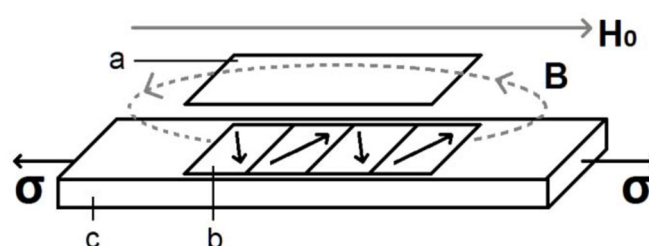
Figure 2. Schematic representation of a wireless strain sensor based on the \Delta E effect: (a) resonator, (b) transducer, and (c) test object. Adapted from [22].
