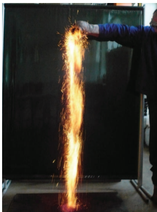
FIGURE 1 Nanoscale zero-valent iron ignites spontaneously when it comes into contact with air.
