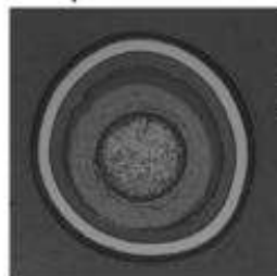
AGR-1 LEU (19.8% U 235 ) TRISO-coated Uranium Oxy-Carbide 12% FIMA burnup
