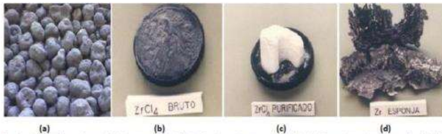
Fig. 2 - Achieved products: (a) Green pellets; (b) Crude zirconium tetrachloride; (c) Pure zirconium tetrachloride; (d) Zirconium sponge [4].
