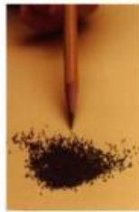
TRISO Coated Particles
