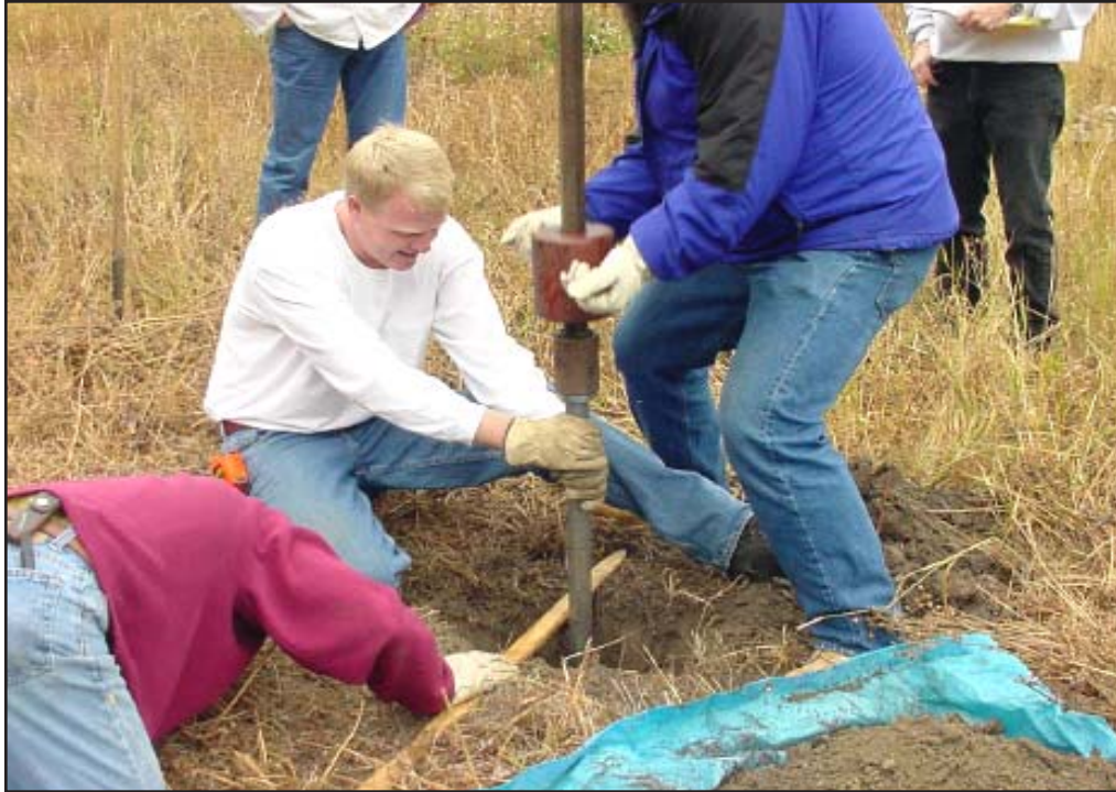
PP testing in progress. Lathe is used to mark the surface of the test hole excavation. In this instance, one person is steadying the equipment, another is lifting and dropping the 35 lb weight, and a third is observing downward displacement and counting blows.
