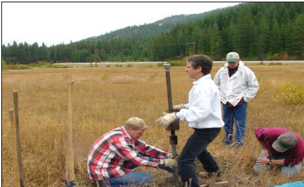
This PP testing can be tiring. Photo shows another person providing relief for the falling weight task.
