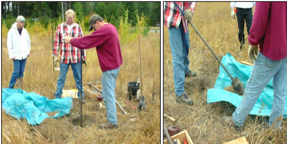
The vicinity of the test hole is cleared of vegetation using a shovel or posthole digger. Left photo shows using the auger to advance the hole to the desired depth. Right photo shows placing soil on the tarp prior to sampling.
