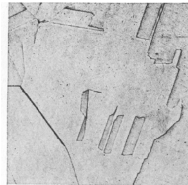
FIG. 4-13. Same as Fig. 4-12, homogenized by heat treatment just below the eutectic temperature and quenched to room temperature; only the silver-rich solid solution is present in this structure. Magnification 100.
