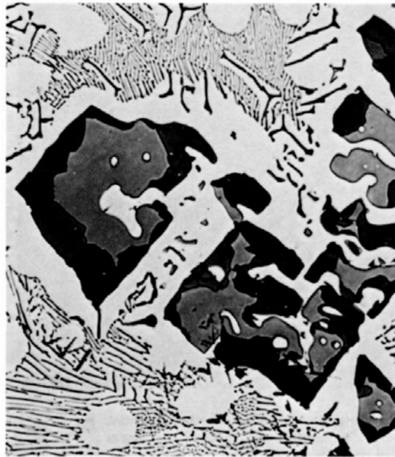
Fig. 3 Primary UAl 3 (gray) partially surrounded by peritectically formed UAl 4 (dark) in an Al-6U alloy that was cooled slowly from above liquidus to 760 °C (1400 °F) and held 10 min, then cooled to 670 °C (1240 °F) and held 15 min (peritectic temperature: 732 °C, or 1350 °F). The matrix is aluminum (white) with UAl 4 (dark) eutectic. This UAl 3 + Al → UAl 4 reaction leads to unfavorable rolling behavior. Electrolytically polished, etched in 50% HNO 3 . 700×
