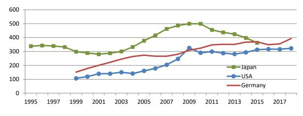
Figure 3: Stock of industrial robots in the automotive industry per thousand blue-collar workers in Germany, the United States, and Japan, 1995–2018 (assumption: Two-shift system)
