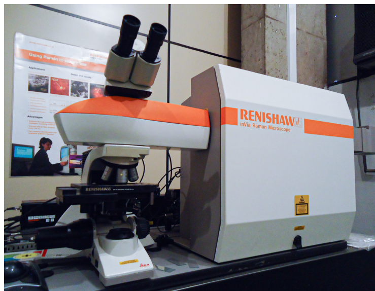
Figure 10 – Raman microscope used in this study's Raman analysis. Photo by the authors.
