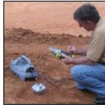
TDR Measurement in-situ
