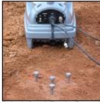
Probes in Ground (Template Removed)
