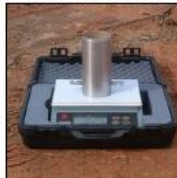
Determine Wet Density
