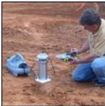
TDR Measurement in Mold
