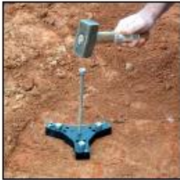
Template for Positioning Probes
