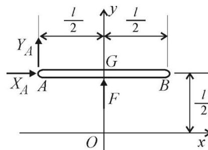
$$\text{TQMA: } \vec{H}_G = J_G \vec{\omega} \Rightarrow \dot{\vec{H}}_G = \frac{ml^2}{12} \alpha \vec{k} = \vec{M}_G = -Y_A \frac{l}{2} \vec{k} \Rightarrow Y_A = -\frac{ml}{6} \alpha \quad (3)$$
