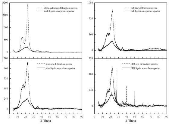
Fig. 2. Comparison of cellulose crystalline structure in alpha-cellulose, oak wood, pine wood, and EFB before and after hydrolysis.
