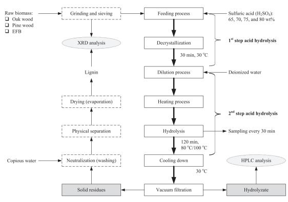
Fig. 1. Overall experimental process stages of the two-step concentrated acid hydrolysis.
