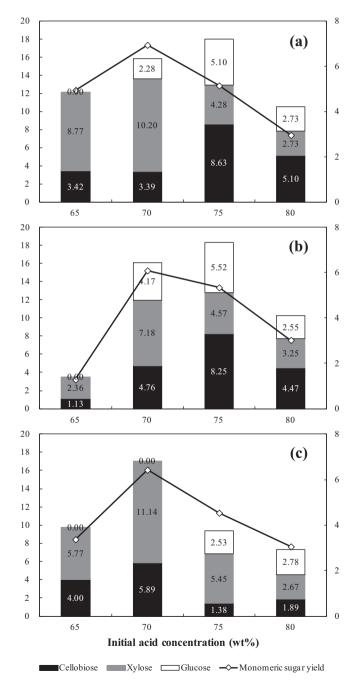
**Fig. 3.** Product distribution at the end of decrystallization reaction from: (a) oak wood, (b) pine wood, (c) EFB, at various initial acid concentration. The primary and secondary vertical axis represents sugar concentration (g/L) and monomeric sugar yield (wt%), respectively.
