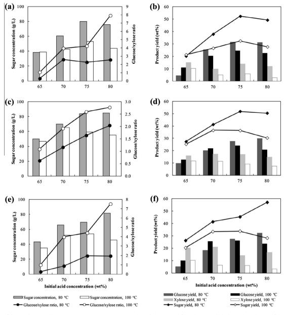
Fig. 4. The effect of decrystallization acid concentration on sugar concentration, glucose/xylose ratio (left), and sugar yield (right) in the hydrolysis of: (a and b) oak wood, (c and d) pine wood, (e and f) EFB, at various hydrolysis temperature.
