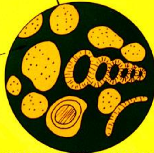
INTERGRANULAR POROSITY FORMED BETWEEN GRAINS.
