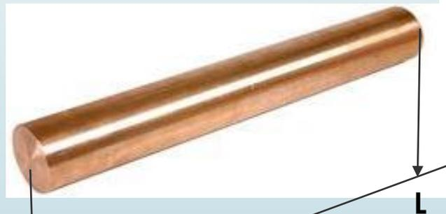
$$\frac{\partial}{\partial x} \left( k \frac{\partial T}{\partial x} \right) + \dot{q}_g = \rho c_p \frac{\partial T(x,t)}{\partial t}$$
