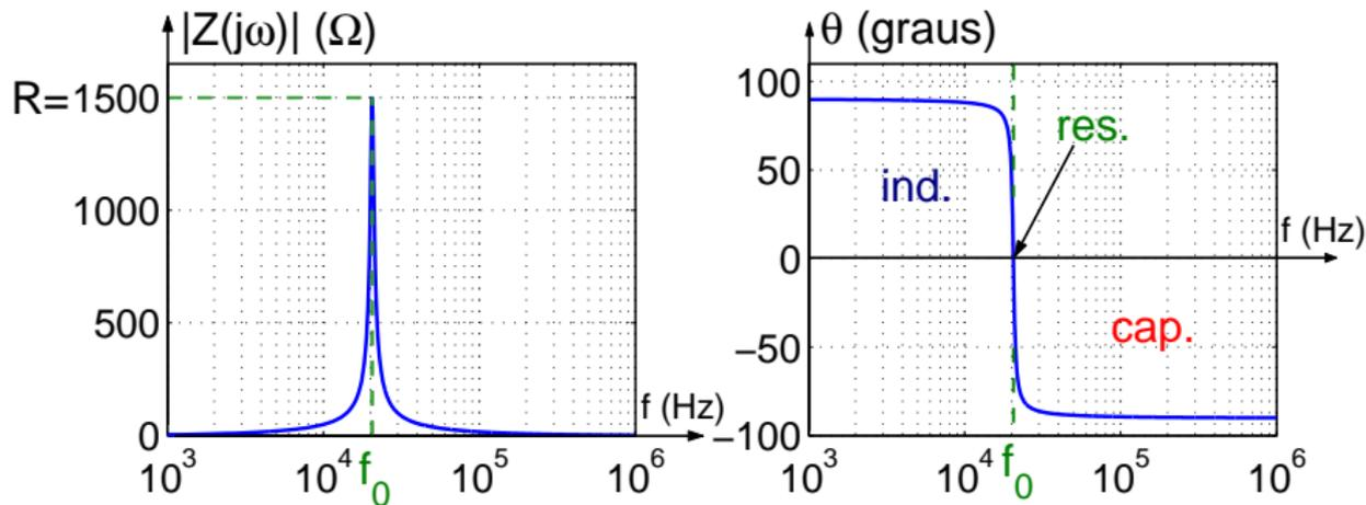
$$\text{Freq. de ressonância: } f_r = f_0 = \frac{1}{2\pi\sqrt{LC}} \approx 20,55 \, \text{kHz}$$
