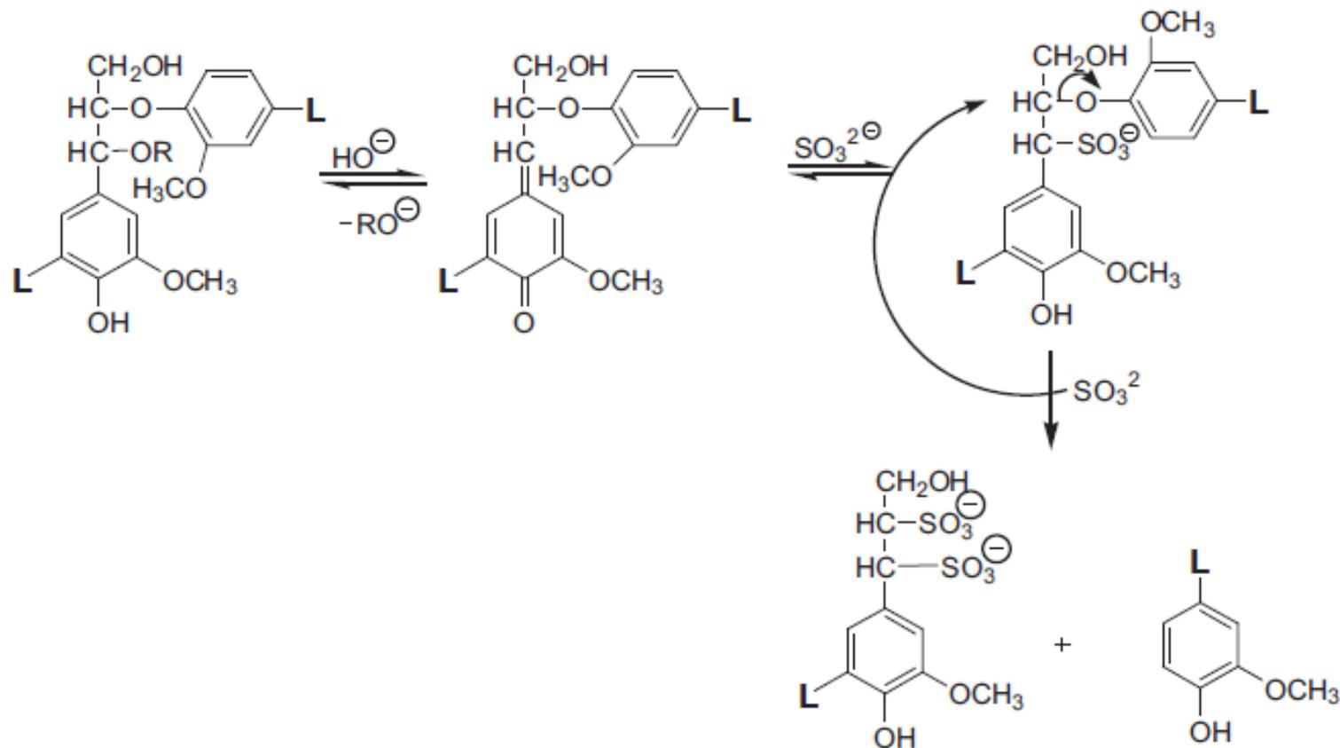
Figure 5.38. Mechanism for the sulphonation of lignin in neutral sulphite pulping.
