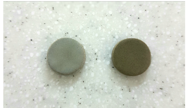
Fig. 12 – Appearance of GC0.29 after immersion in HCl (left) and NaOH (right) solutions for 6 h.
