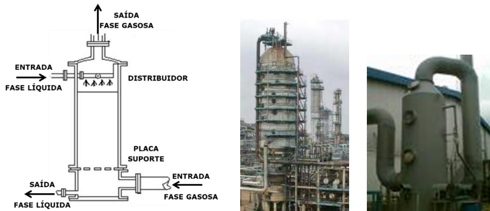
Figura 09 – Torre ou coluna absorvedora (Scrubber)
