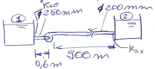
$$\left( \alpha_1 \frac{V_1^2}{2g} + \frac{P_1}{\rho g} + z_1 \right) - \left( \alpha_2 \frac{V_2^2}{2g} + \frac{P_2}{\rho g} + z_2 \right) = \frac{\dot{W}_a}{\rho g Q} - \frac{\dot{W}_m}{\rho g Q}$$
