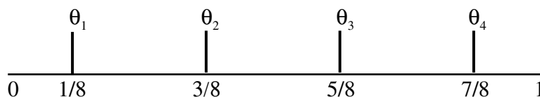
Figure 11.14 Efficient Location N = 4
