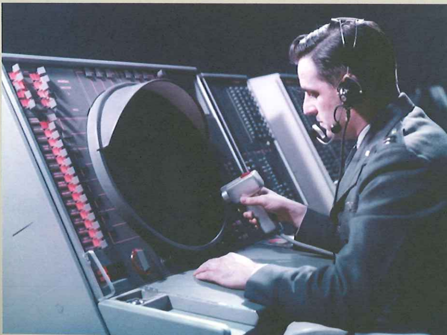
Operator using the SAGE System interface.
