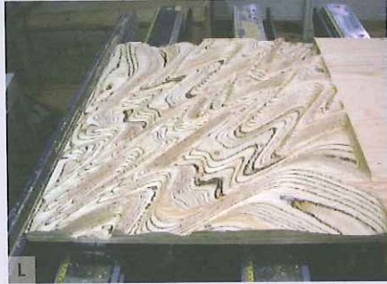
K, L, AND M Milling of mathematical surfaces at end grain of laminated ply.
