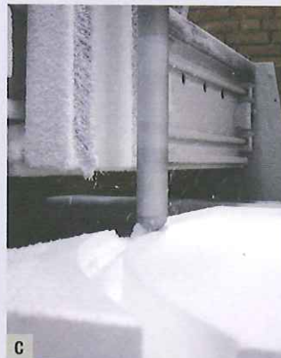
C A CNC milling machine is used to cut expanded polystyrene blocks, which are combined to form molds for different panels.
