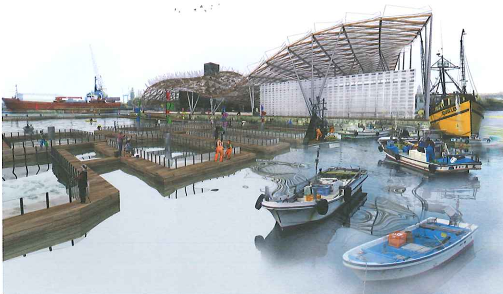
Diagrid roof canopy developed using morphogenetic design principles. For explanation of this process see opposite page.
