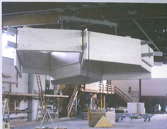
H A full-size prototype of several structural cells allows the designers to inspect the aesthetic and structural characteristics of the roof.
