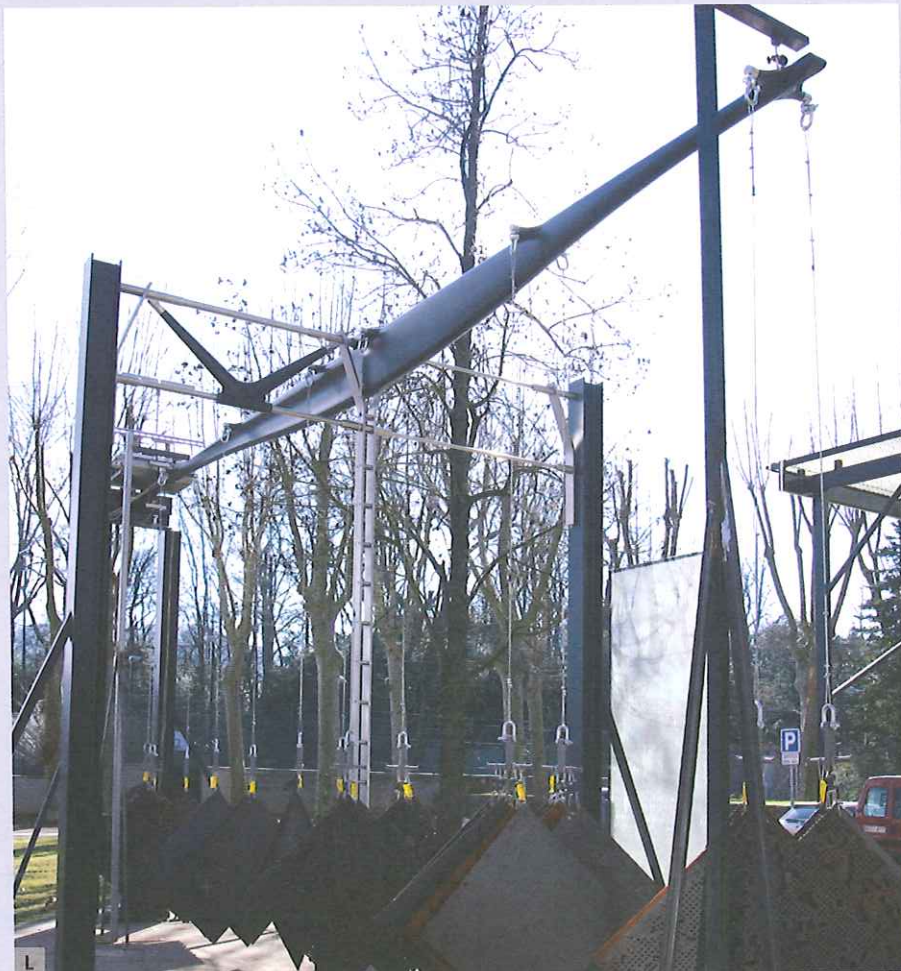
H CNC-milled mold for forming beams.
