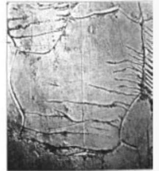
Fig. 12. Same after 40,000 revolutions. \times 1000 .
