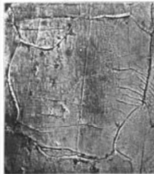
Fig. 11. Same after 10,000 revolutions. \times 1000 .
