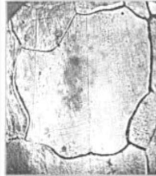
Fig. 9. Specimen after 1000 revolutions of a stress of 17.4 tons per sq. inch. \times 1000 .
