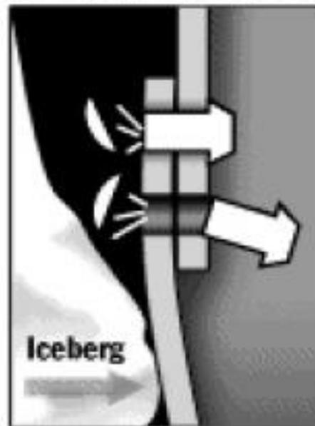
**2.** Pressure from the iceberg collision may have caused the rivets to pop along some hull plates, causing the seams to open.
