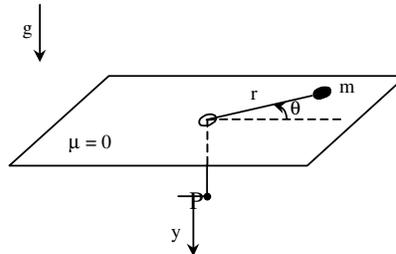
Resp.:  $(R - v_0 t)\ddot{\theta} - 2v_0\dot{\theta} = 0$        $\dot{\theta} = \frac{R^2 \omega_0}{(R - v_0 t)^2}$
