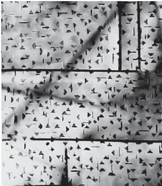
Figure 11.1. Nuclei of Cu_2O formed on copper surface at 10^{-1} mmHg oxygen pressure (13.3 Pa), 525^\circ C , 20 s (17,600 \times ). Black lines are bands of imperfections (stacking faults) in the copper lattice (Brockway and Rowe [5]).
