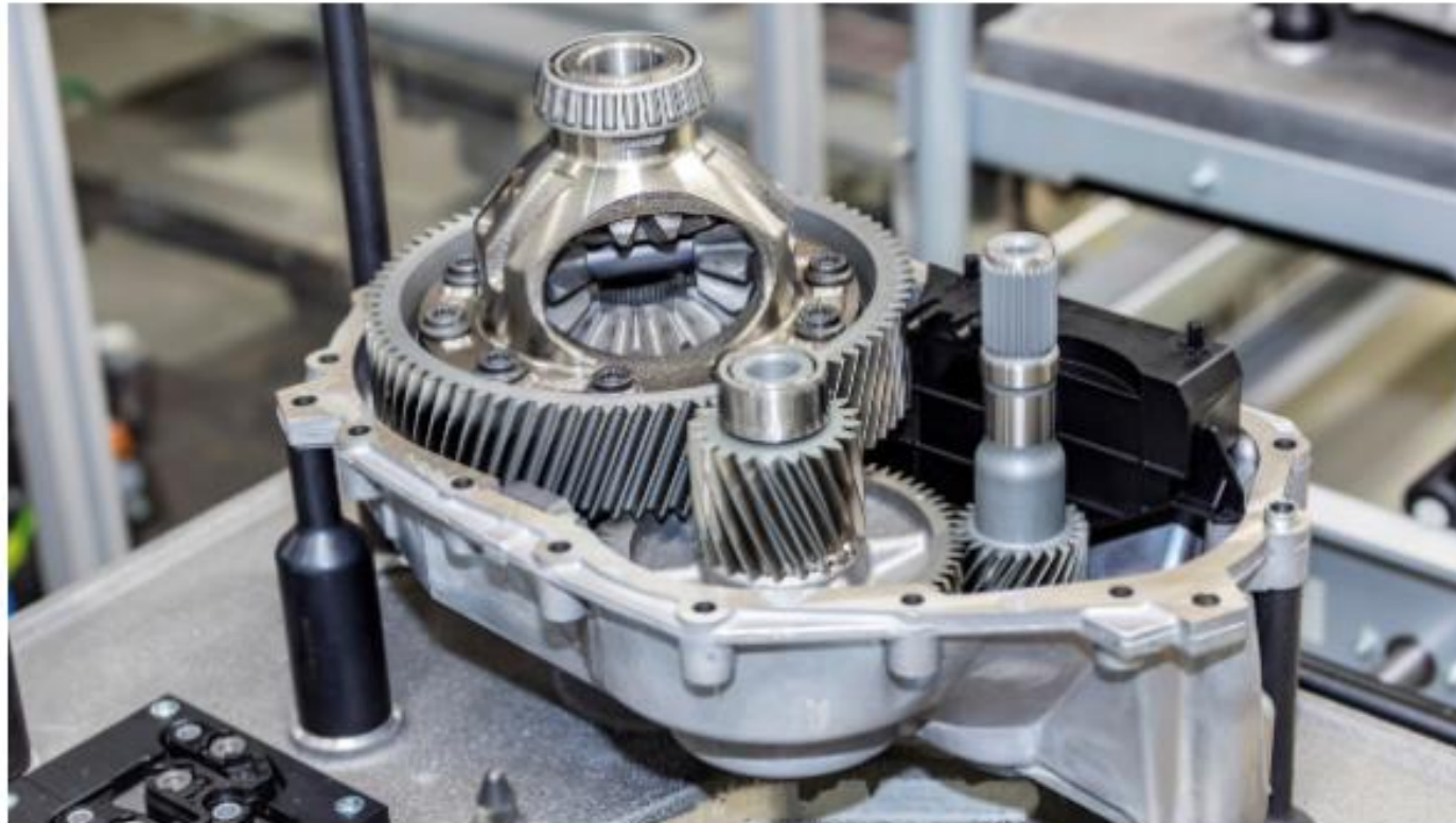
Small shifting unit: the 1-speed gearbox
