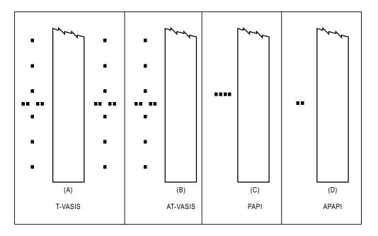
Figure 5-15. Visual approach slope indicator systems
