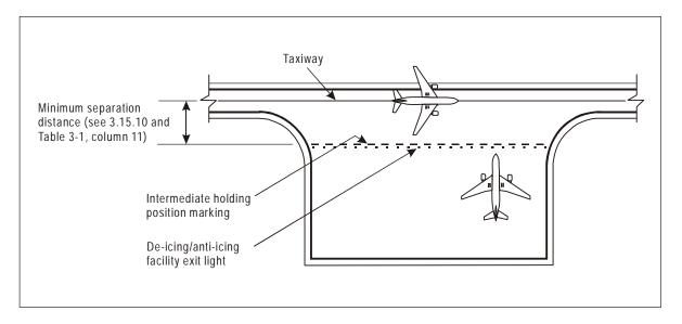
Figure 5-26. Typical remote de-icing/anti-icing facility
