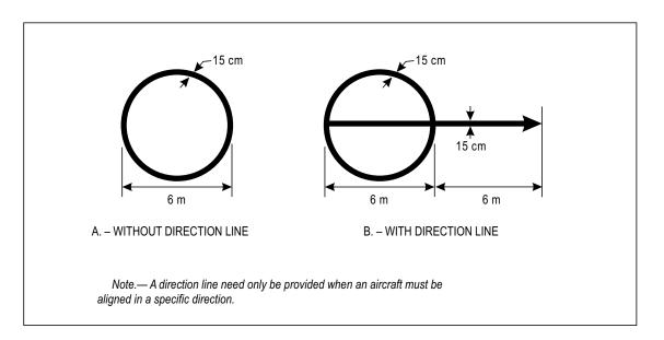
Figure 5-8. VOR aerodrome check-point marking
