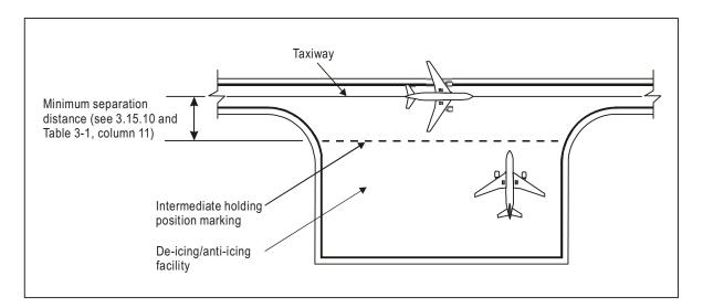
Figure 3-4. Minimum separation distance on a de-icing/anti-icing facility
