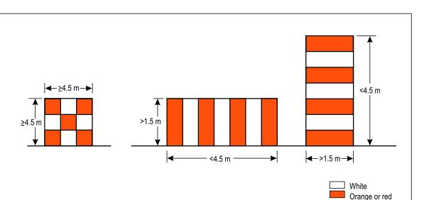
Figure 6-1. Basic marking patterns
