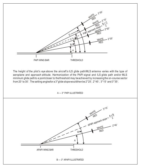
Figure 5-19. Light beams and angle of elevation setting of PAPI and APAPI
