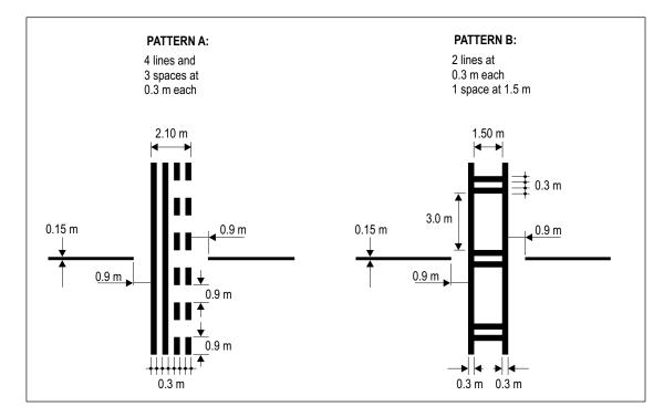
Figure 5-7. Runway-holding position markings
