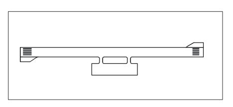
Figure 3-1. Typical turn pad layout
