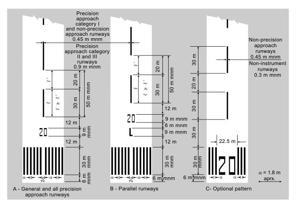
Figure 5-2. Runway designation, centre line and threshold markings
