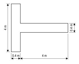
Figure 5-1. Landing direction indicator
