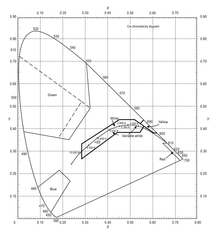
Figure A1-1. Colours for aeronautical ground lights
