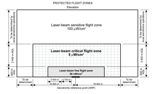
Figure 5-12. Protected flight zones with indication of maximum irradiance levels for visible laser beams
