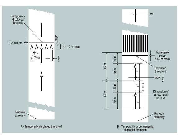
Figure 5-4. Displaced threshold markings
