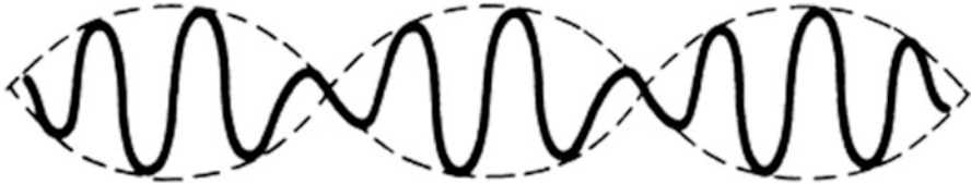
Fig. 4.1 Spatial variation of the electric field of two waves with a frequency difference
