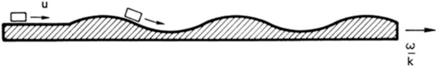
Fig. 7.22 Mechanical analogy for an electron moving in a moving potential
