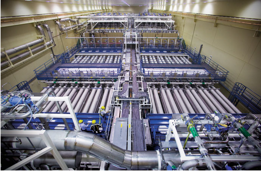
Fig. 10.60 The laser bay of the National Ignition Facility [courtesy of Lawrence Livermore Laboratory via Google Images]
