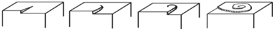
Figure 5.5 A screw dislocation that generates a growth spiral (Mullin, 2003). Copyright Wiley-VCH Verlag GmbH & Co. KGaA. Reproduced with permission.
