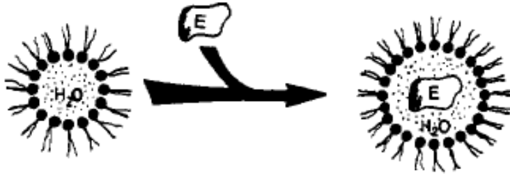
Figure 1. Schematic representation of the solubilization of enzymes in reverse micelles (cross section) and of the structure of the surfactant AOT used in our studies. Particularly at small w_o values ( w_o = [\text{H}_2\text{O}]/[\text{AOT}] ) the uptake of the material present
