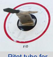
Pitot tube for <u>Airbus A380</u>, together with an <u>angle-of-attack</u> vane (left). Air-flow is right to left.
