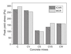
Fig. 4. Comparative results between the Germann ICiAR rheometer and Physical MCR501 rheometer [59].
