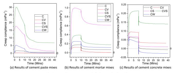
Fig. 10. Creep and creep recovery test results for the cement-based materials.
