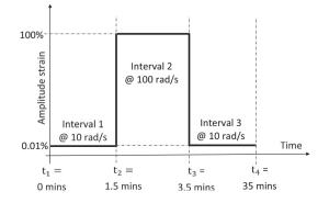
Fig. 7. Schematic test protocol for the 3ITT thixotropy test.
