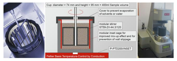
Fig. 2. Special building material cell (BMC 90) [46] and MCR 501 rheometer.
