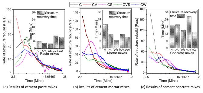
Fig. 15. Rate of restructuration and structure recovery time.
