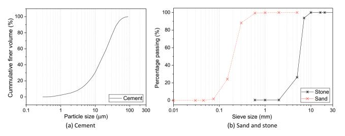
Fig. 3. Particle size distribution of the dry constituents.
