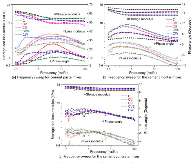
Fig. 9. Frequency sweep results of the cement-based materials.
