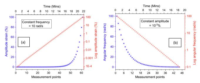
Fig. 5. Test protocol for the (a) amplitude sweep (b) frequency sweep.
