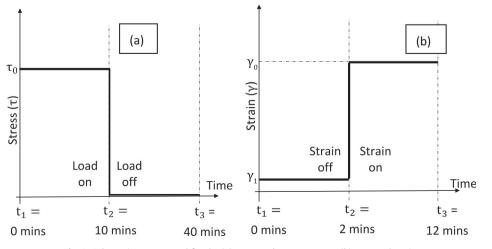
Fig. 6. Schematic test protocol for the (a) creep and creep recovery (b) stress relaxation.
