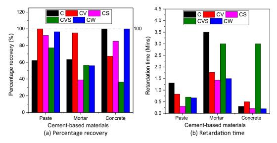
Fig. 11. Percentage recovery and retardation time of the cement-based materials.
