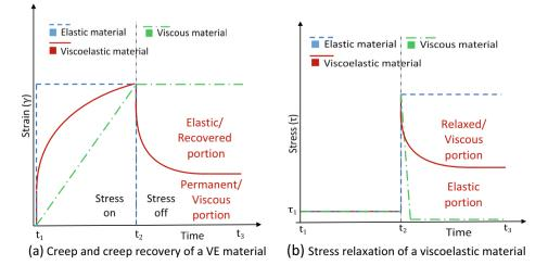
Fig. 1. Viscoelastic behaviour/response to a sustained shear strain and stress.
