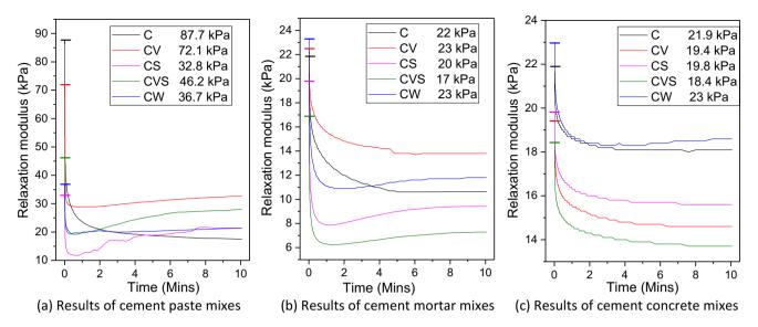
Fig. 12. Stress relaxation test results for the cement-based materials.
