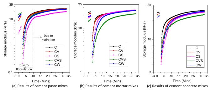
Fig. 14. Three interval thixotropy test results for the cement-based materials.
